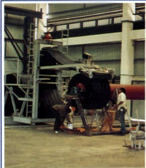
CBI Overseas Inc. (CBIO) offers design and supply of rotating biological contactors (RBC's) commonly used for biological removal of carbonaceous BOD. CBIO operates with technical support from CBI Walker, Inc. (USA) and manufactures the units (known as the "BioWrap") at its Singapore facility. The "BioWrap" is specifically designed to provide superior structural characteristics while offering enhanced process performance through a unique spirally wound media arrangement.
